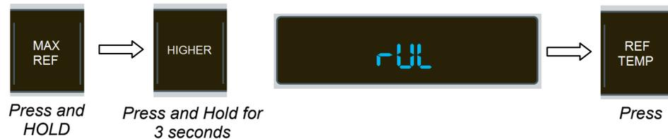
To access the Fresh Food (*on some models*) lower temperature limit, Press and HOLD the **MAX REF** button. While holding the **MAX REF** button, press the **LOWER** pad and HOLD for 3 seconds until **rLL** is shown in the display. Depress the **REF TEMP** pad to display the default setting.
