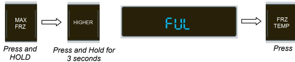
To access the Freezer (*on some models*) lower temperature limit, Press and HOLD the **MAX FRZ** button. While holding the **MAX FRZ** button, press the **LOWER** pad and HOLD for 3 seconds until **FLL** is shown in the display. Depress the **FRZ TEMP** pad to display the default setting.
